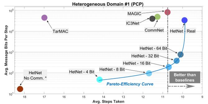
**Figure 4: Communicated bits per round of communication vs. performance in PCP for different methods. HetNet facilitates binarized messages among agents which requires significantly less CB as compared to real-valued baselines.**
