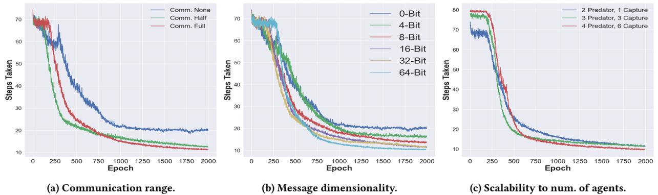
**Figure 5: Analyzing HetNet’s performance with and without communication (Fig. 5a) and across different binary message dimensions (Fig. 5b) in the PCP domain. Communication policy learned by HetNet improves the cooperativity among agents and the performance improves with larger message sizes. Fig. 5c depicts results for analyzing HetNet’s ability to scale to different number of agents. As shown, HetNet-Binary can successfully scale to different sizes of the composite team.**
